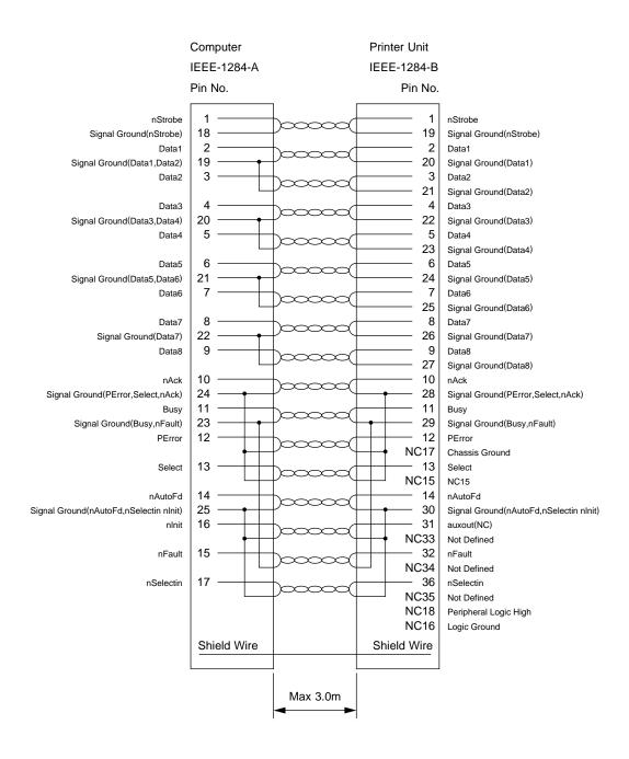
NOTE: The printer cable must be shield-structured.
